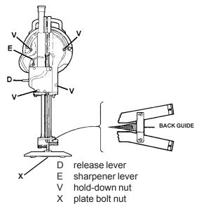
Figure 3. Removing the Sharpener
