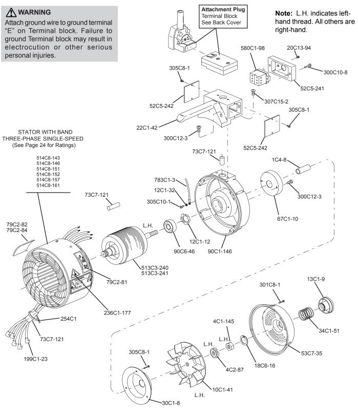
Figure 24. Three-Phase Motor Assembly (Exploded View)
