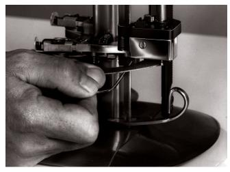
Figure 9. Adjusting Bevel Bloc Shoes
