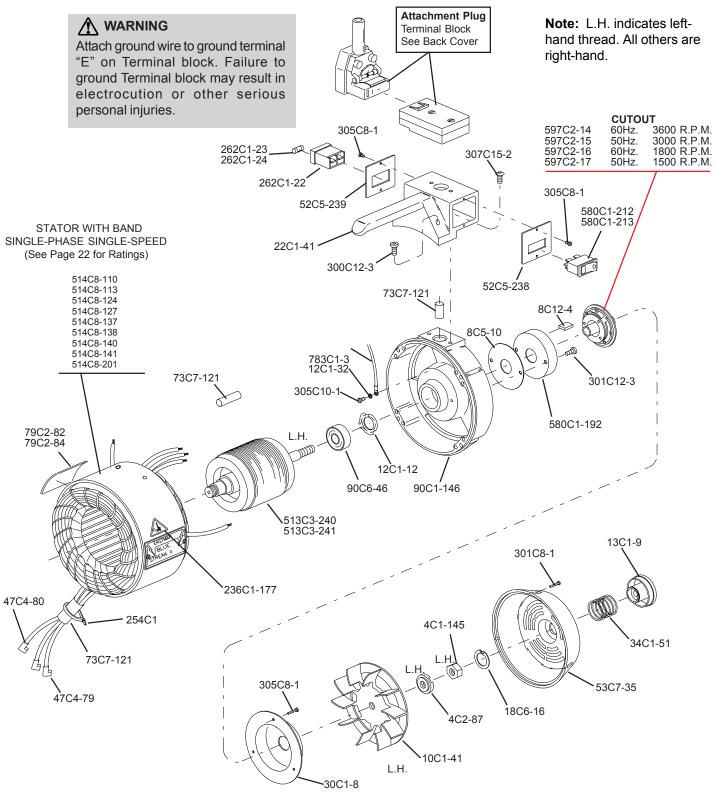
Figure 22. Single Phase Motor Assembly (Exploded View)
