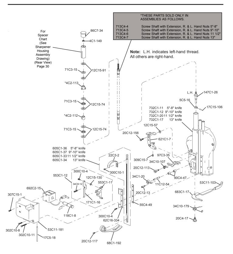
Figure 27. Sharpener Housing Assembly (Exploded, Front View)
