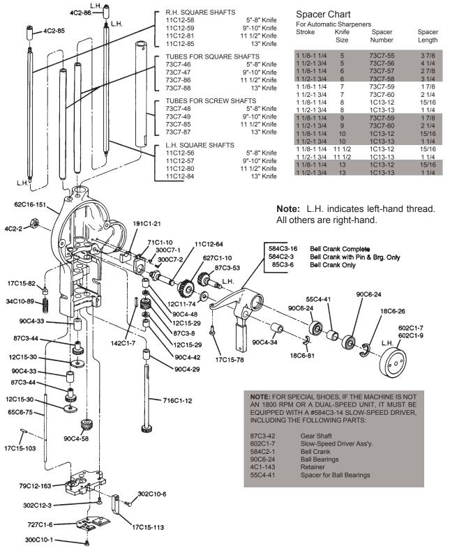
Figure 29. Sharpener Housing Assembly (Exploded, Rear View)
