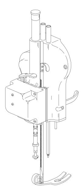
Figure 26. Sharpener Housing Assembly (Assembled, Front View)
