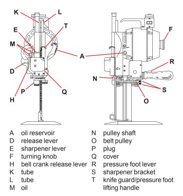
Figure 2. Controls and Adjustments
