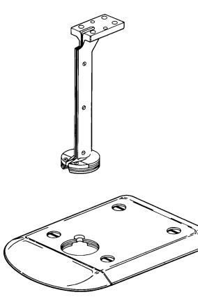
Figure 32. Standard and Baseplate Assembly (Assembled View)
