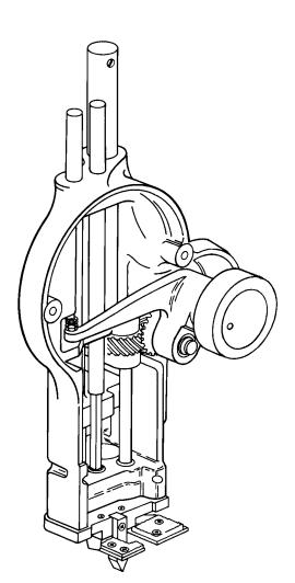
Figure 28. Sharpener Housing Assembly (Assembled, Rear View)
