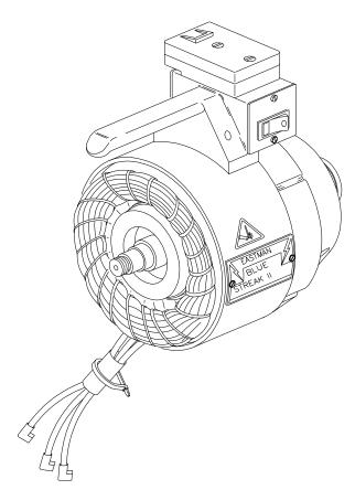
Figure 21. Single-Phase Motor Assembly (Assembled View)
