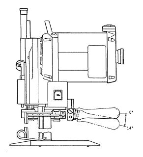
Available as an option on new machines or for retrofitting to any existing Eastman straight knife, the Ergo-Handle allows the operator to adjust the handle downward from the standard horizontal through a 14-degree range. Adjusting the handle's angle to suit the operator's preference allows for more effective use of the arm muscles, while placing less strain on the wrist and thumb.
