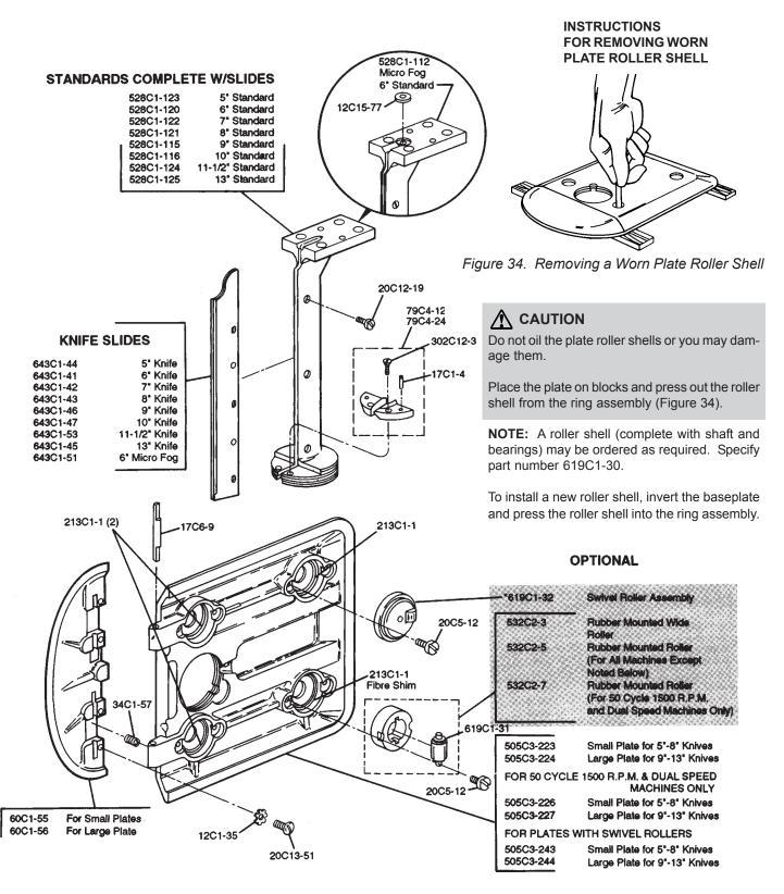
*Figure 33. Standard and Baseplate Assembly (Exploded View)*
